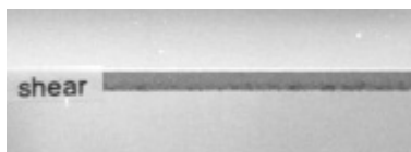
Droop after shear cutting
